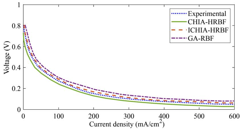
Fig. 6. Current-voltage curve validation for the achieved method based on DCHIA-HRBF and other comparative algorithms for  $T=1173.15\text{ K}$
