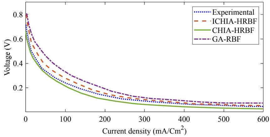
Fig. 4. Current-voltage curve validation for the achieved method based on DCHIA-HRBF and other comparative algorithms for  $T=873.15\text{ K}$
