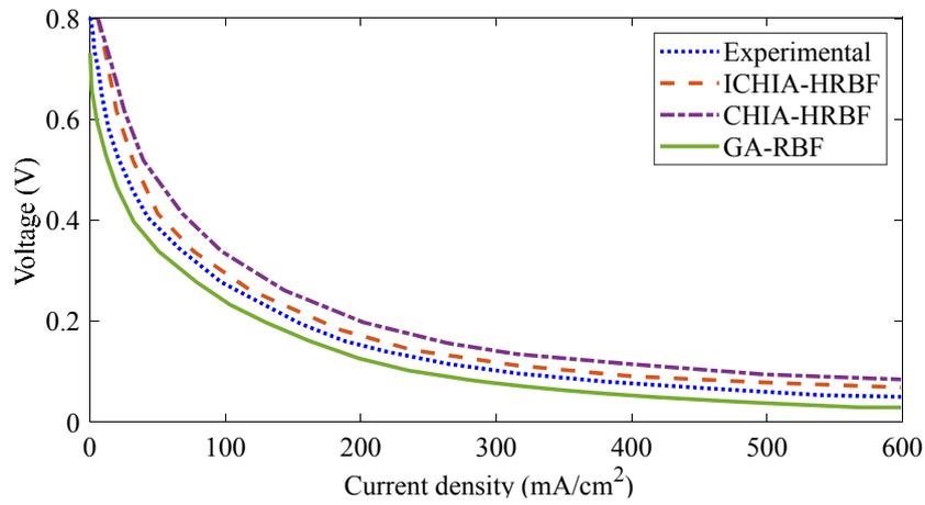
Fig. 5. Current-voltage curve validation for the achieved method based on DCHIA-HRBF and other comparative algorithms for  $T=1223.15\text{ K}$
