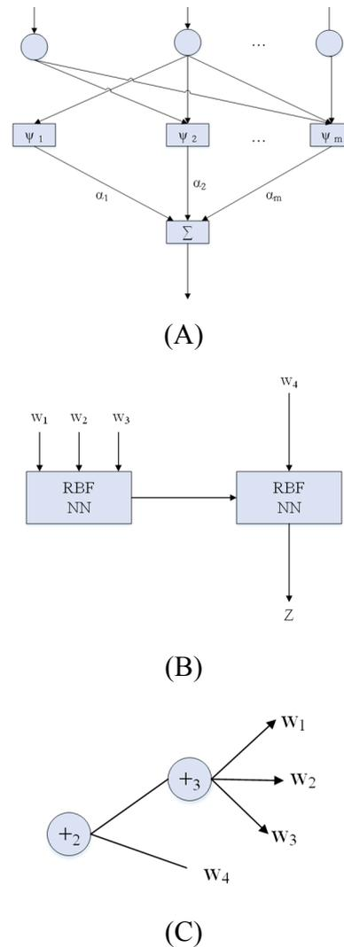
Fig. 1. (A) basic RBF network, (B) HRBF network, and (C) tree-structural HRBF network
