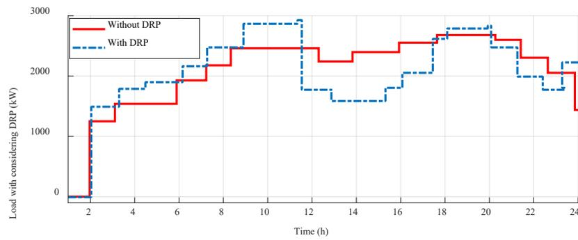
Fig. 8. The profile of the power generation with and without DRP based on interval PSO algorithm
