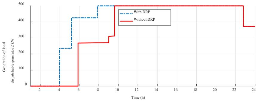
Fig. 14. The profile of power generation of LDG2 with and without DRP based on interval PSO algorithm
