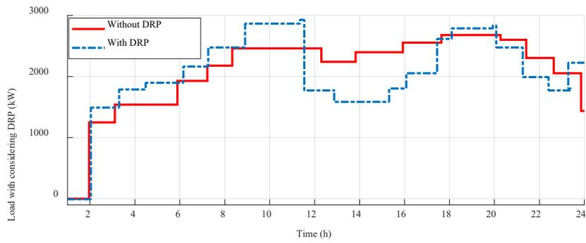
Fig. 6. The energy demand with and without DRP based on Interval PSO algorithm
