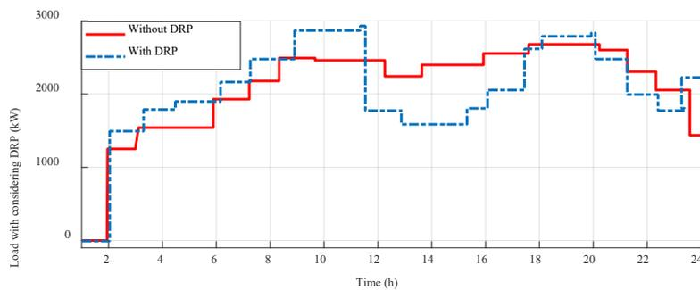
Fig. 5. The energy demand with and without DRP based on the deterministic method
