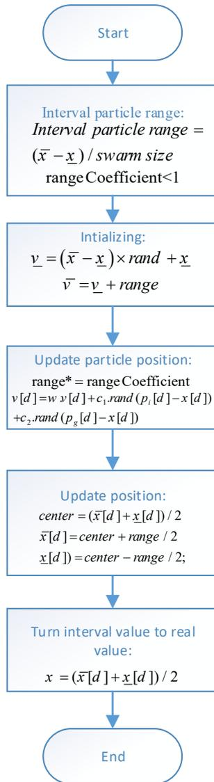
Fig. 2. The flowchart diagram of interval PSO algorithm
