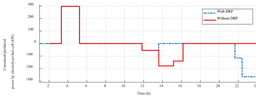
Fig. 17. The Charge/discharge profile of the hydrogen storage system with and without DRP by the deterministic method
